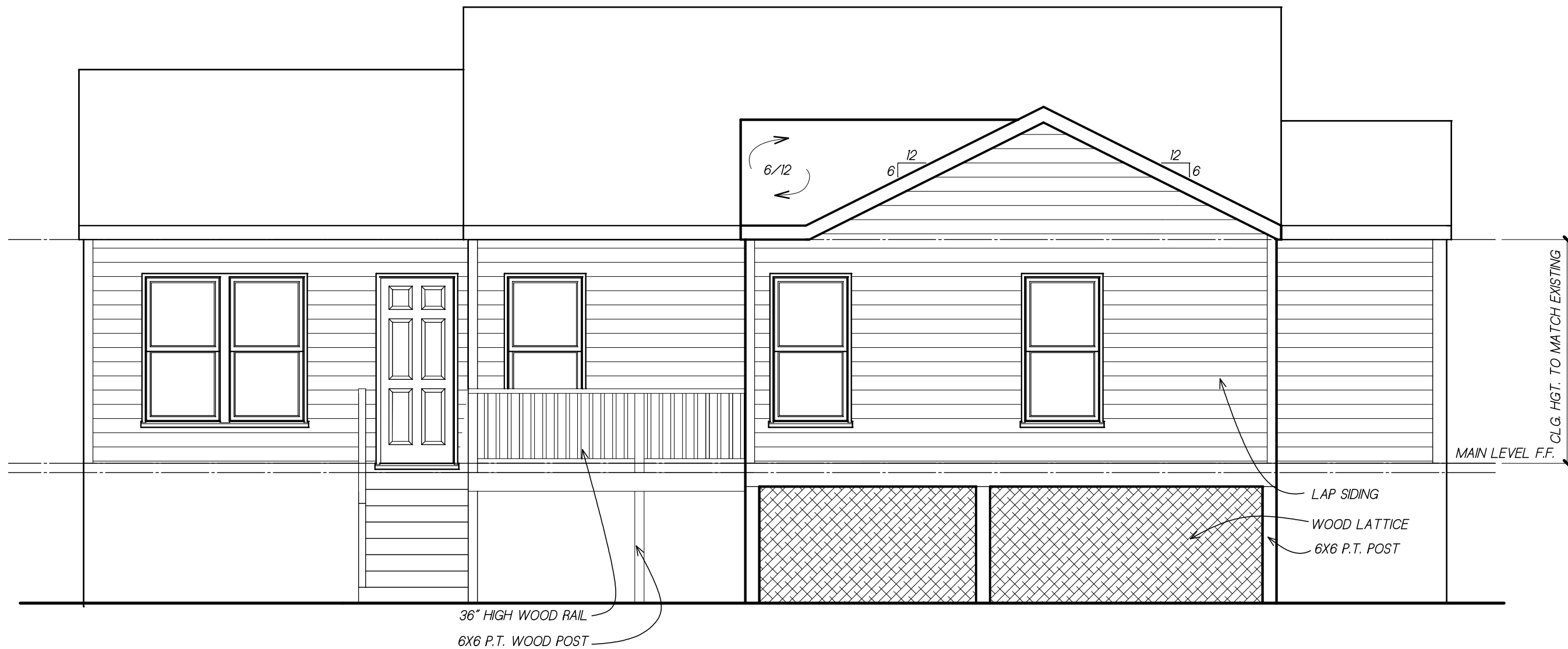
PROPOSED REAR ELEVATION 2 A9 SCALE: 1/4" = 1'-0"
